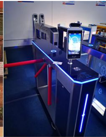
Temperature detector integrated with turnstile
