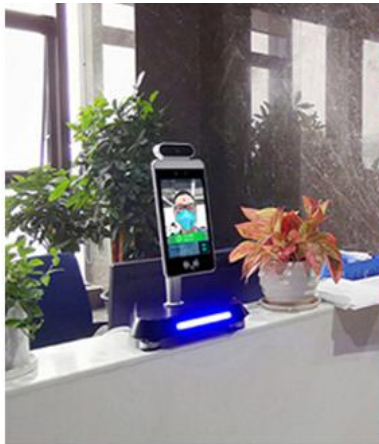
Temperature detector with desk type bracket
